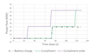
Fig. 5. Control with constant generation and load, one overload
