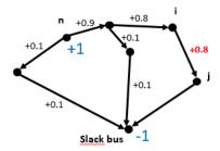
Fig. 1. Example of PTDF on a small network
